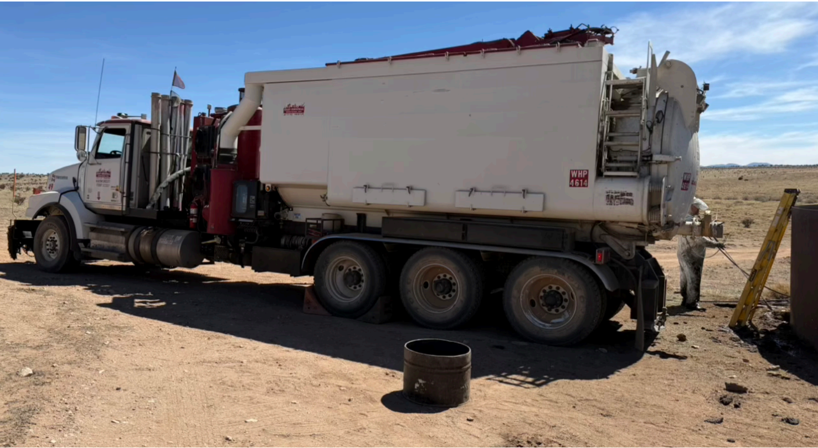
The slurry truck uses high volume suction to remove debris from the tank and transfer it to the truck's holding tank.
